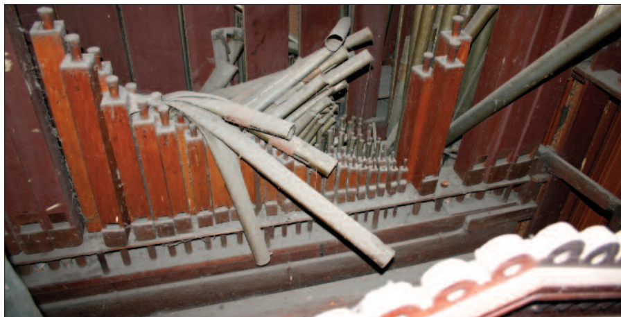
Fig. 16. Busby, 19 August 2008: The soot-covered wooden and collapsed metal pipes of the 'Choir' and 'Swell' pipes poking between the vertical shutters. Pipe-metal (a tin-lead alloy) is very soft and the collapse of a few taller pipes evidently had a disastrous 'knock-on' effect!
